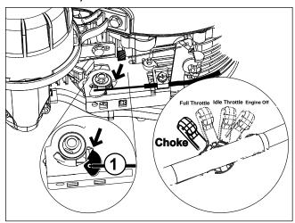
Following these steps for the throttle adjustment will ensure that the Kawasaki engine performs properly for this mower. The engine speed is adjusted to approximately 3600 RPM at the factory.
