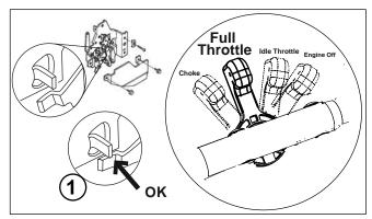
Following these steps for the throttle adjustment will ensure that the Honda engine performs properly for this mower. The engine speed is adjusted to approximately 3600 RPM at the factory.
